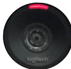
In smaller rooms with a Logitech Meetup camera a red light will appear on the camera to signify that the microphone is muted as illustrated to the right. A mute icon is displayed on the TV Screen for all devices.
